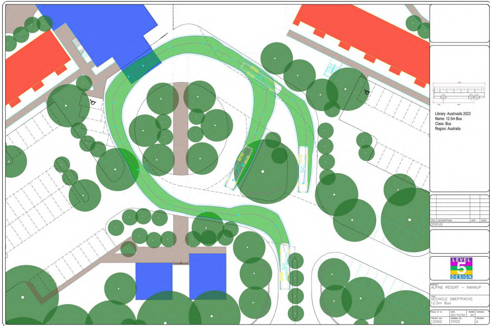
12.5m Bus Internal Manoeuvring
