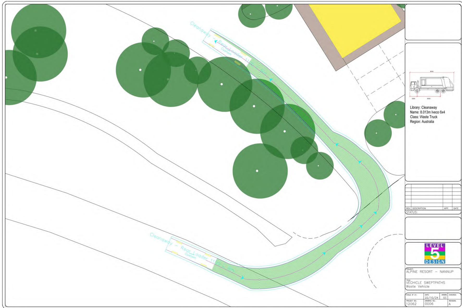
Waste Vehicle Access
