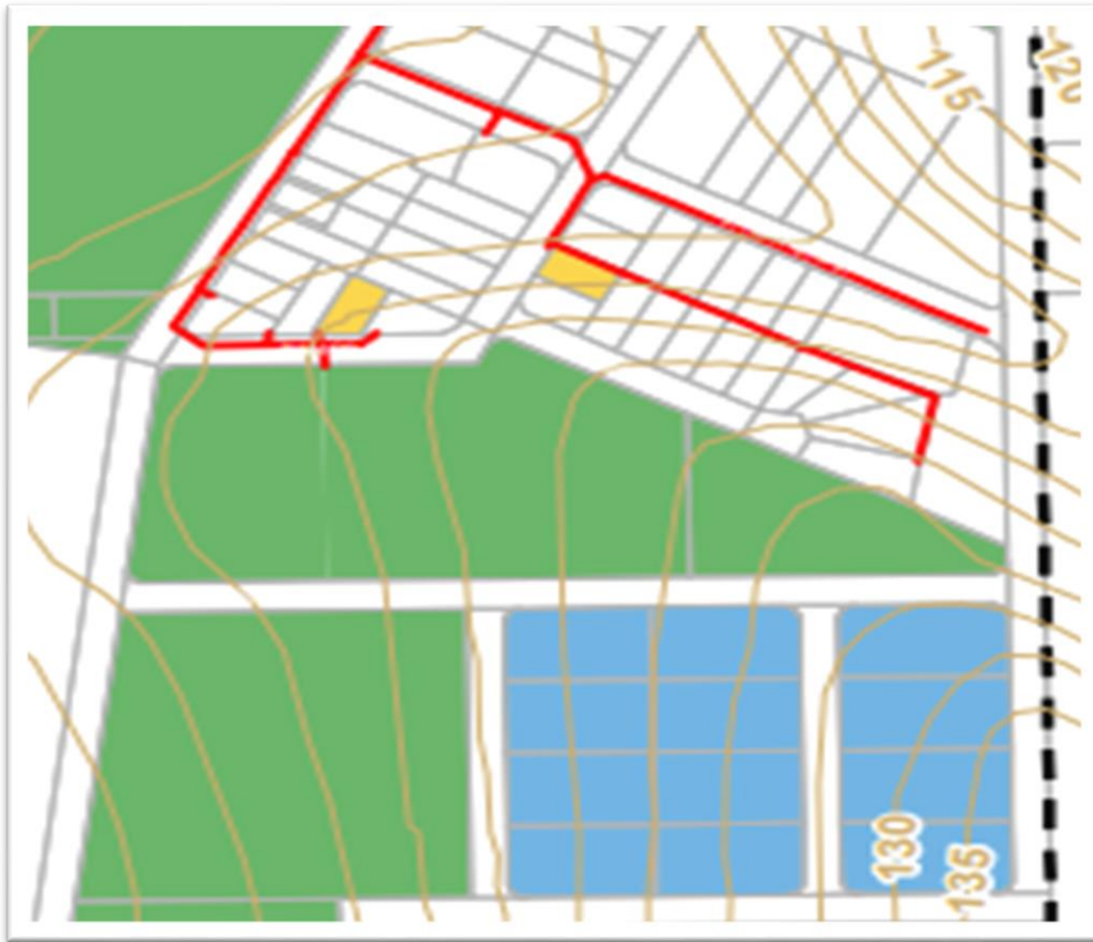
Figure 3 – Current Deep Sewerage Map
