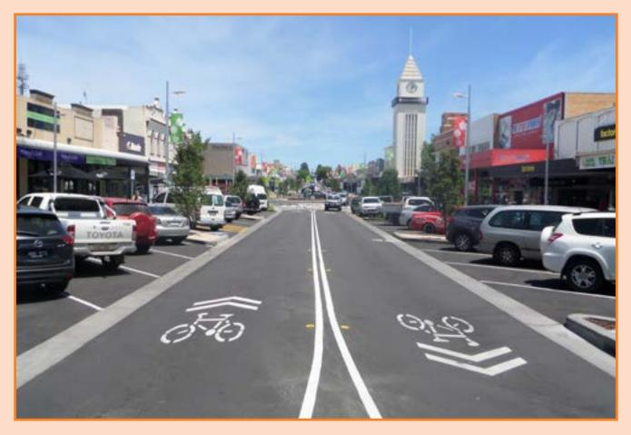
Figure 4.17 Shared-lane markings, traffic calming and lower posted speed limits have improved cycling safety through Warrnambool's town centre in regional Victoria.
